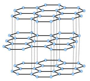
Graphite has very strong bonds *within* the layers of carbon atoms but much weaker bonds *between* the layers. This allows the layers to slide past one another quite easily, which accounts for graphite's slipperiness.
